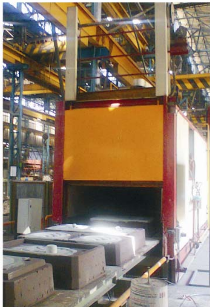
Hot Air Impingement Dryer for Moulds in Foundry Industry
