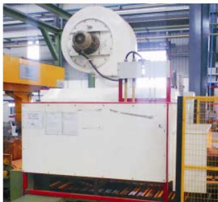
IR Pre-Dryer Oven in Mould Painting Line
