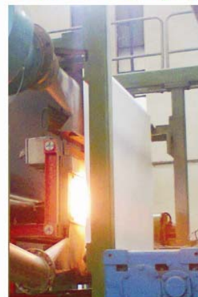
High intensity IR dryer for coating immobilisation
