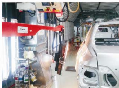
IR Touch-up Paint Curing
