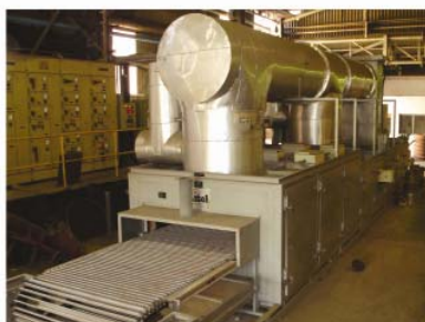
IR Convection Oven for Core Drying in Foundry
