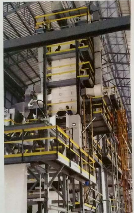
Tower dryers for Glass-fibers / Teflon curing / Tyre cords
